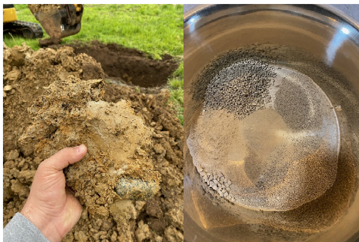
Figure 1 (Left): Wet soil sample from the Lone Pine Medical Facility Project indicates cemented well graded sand rather than Lacamas Silt Loam, Figure 2 (Right): Separated dry soil sample from Lone Pine Medical Facility Project to show soil grain size analysis.
